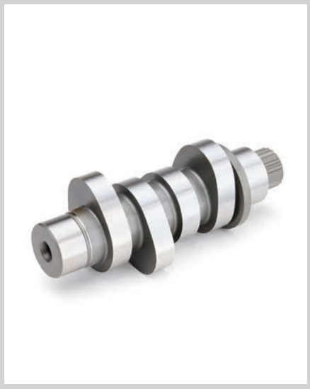
C. SCREAMIN' EAGLE SE8-550 CAM – MILWAUKEE-EIGHT ENGINE
